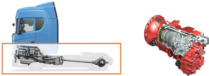
Figure 3. Cutaway illustration of a Corporate A truck powertrain, with a heavy-duty gearbox.
