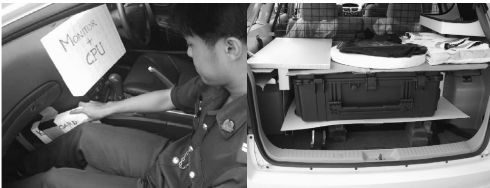
Figure 1. Foam models to explore the positioning of equipment in the front and rear interior of the vehicles
