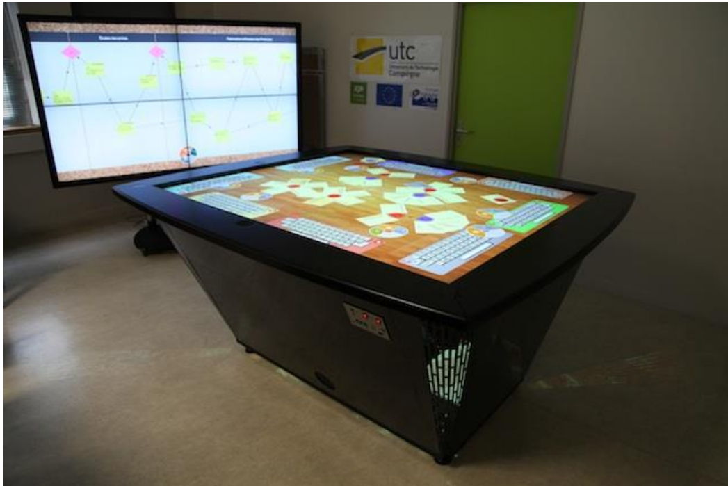
Figure 3. The TATIN-PIC platform, as an example of HOVER platform composed of a Horizontal and vertical interactive surface
