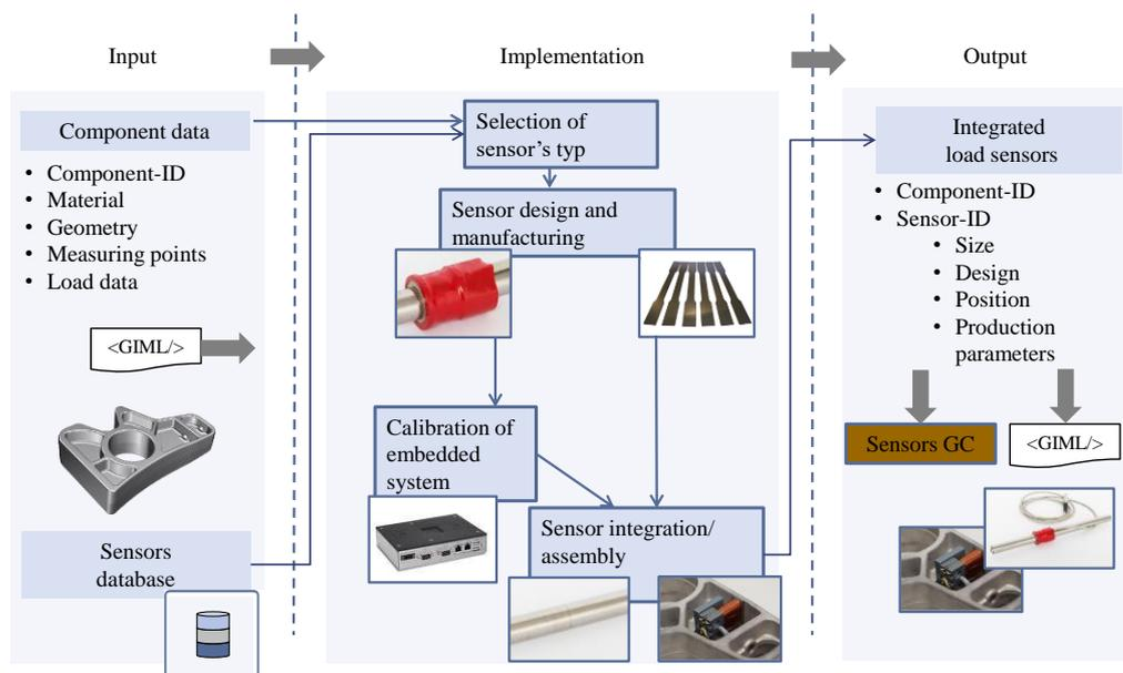
Figure 3. Implementation of Sensors in a Component
