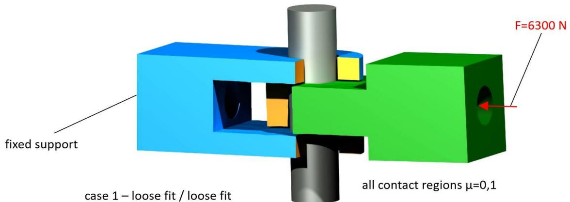
Figure 7. Boundary conditions for the simulation of the non-ideal assembly
