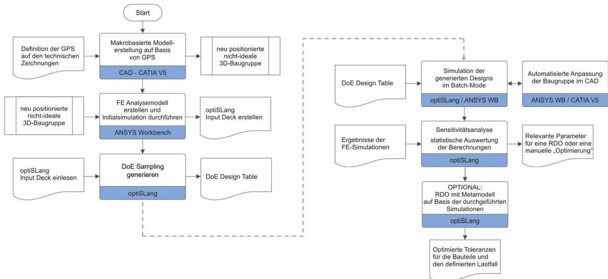
Figure 3. Flowchart of the new geometric tolerance analysis approach
