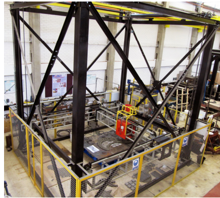
Figure 1. 3D concrete printing machine
