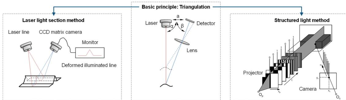
**Figure 3. Functionality of triangulation and usage as laser light section method [Katona et al. 2014b] and structured light method [Gühring 2002]**
