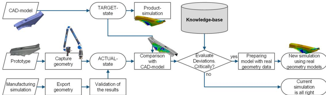
**Figure 2. Desired process for the integration of real geometry data into product simulations**
