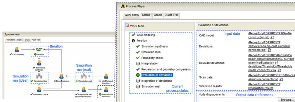
Figure 9. Mapped simulation processes and dialogue component to evaluate and integrate deviations [Kestel et al. 2015a]
