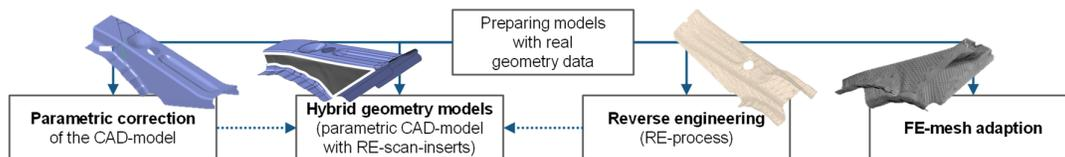
**Figure 5. Provided methods to prepare the model with real geometry data**
