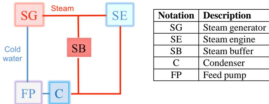
Figure 1. Schematic sketch of the system
