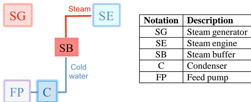
Figure 2. Schematic sketch of the system during discharge
