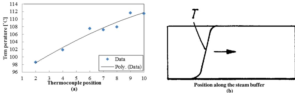
Figure 10. Temperature gradient along the buffer for the discharging phase as obtained (a) experimentally and (b) theoretically [1]
