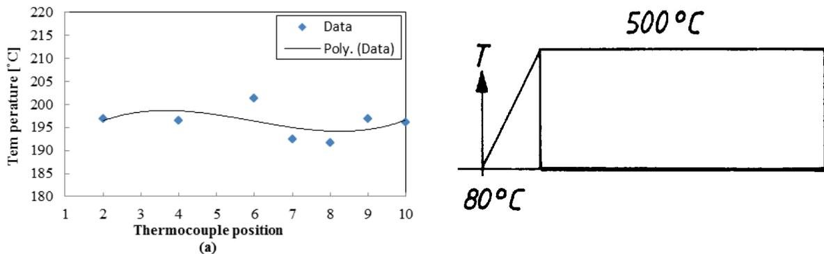
Figure 9. Temperature gradient along the buffer as it is fully charged as obtained (a) experimentally and (b) theoretically [1]
