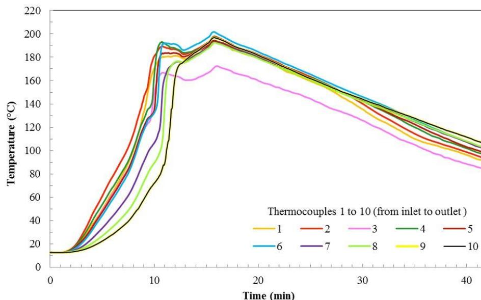
Figure 7. Temperature profile of each thermocouple along the steam buffer
