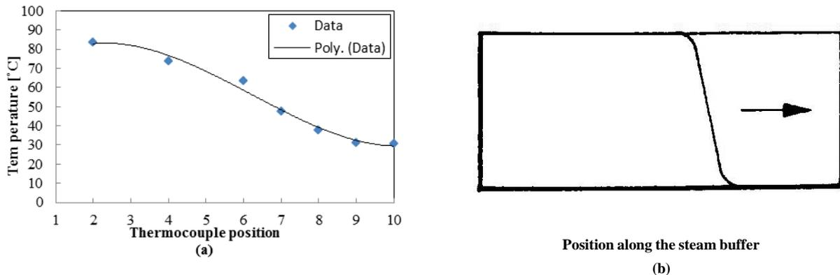
Figure 8. Temperature gradient along the buffer for the charging phase as obtained (a) experimentally and (b) theoretically (edited from [1] to match inlet direction)
