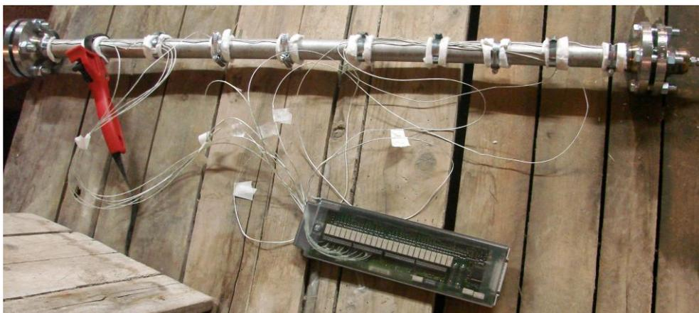
Figure 6. Attachment of the thermocouple wires to the buffer and to the measurement card
