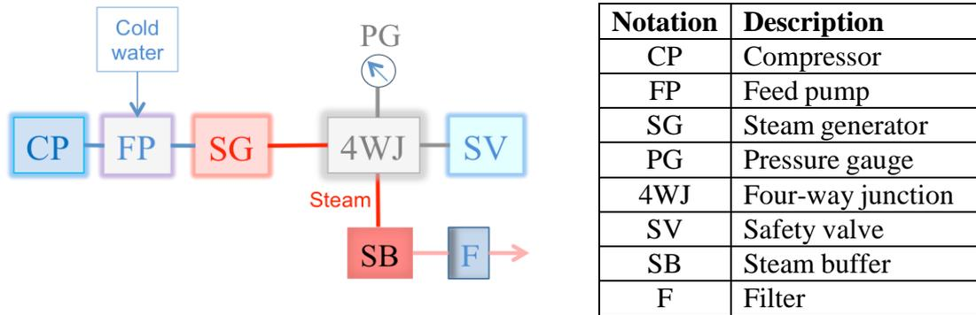
Figure 5. Schematic of the test-rig
