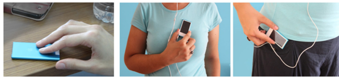
Figure 3. Pausing the song by reversing the music player, changing the place of the device to change the playlist
