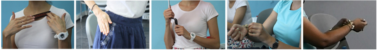
Figure 6. Pausing and playing the song by a tap on the flat necklace, a tap on the skirt, pulling the stripe of an umbrella, stretching the elastic bracelet and leaving it back, and turning the elastic bracelets inwards
