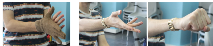
Figure 10. Playing and pausing songs: Gloves sensing the clapping of the hands; the bracelet sensing the muscular movement specific to the each hand gesture that corresponds to play and pause in order, from left to right
