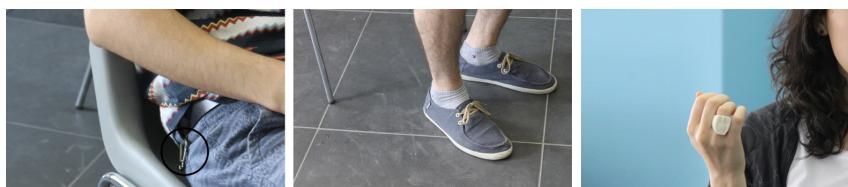
Figure 13. Controls through foot gestures tracked by the clip attached to the pants and controls through proximity of jewellery pieces
