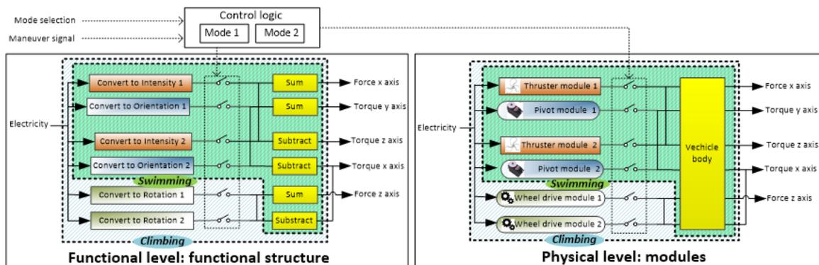
Figure 7. The modular architecture of the Searazor prototype
