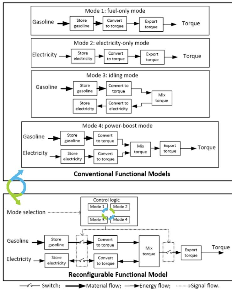
Figure 1. The reconfigurable functional model that operates in four modes
