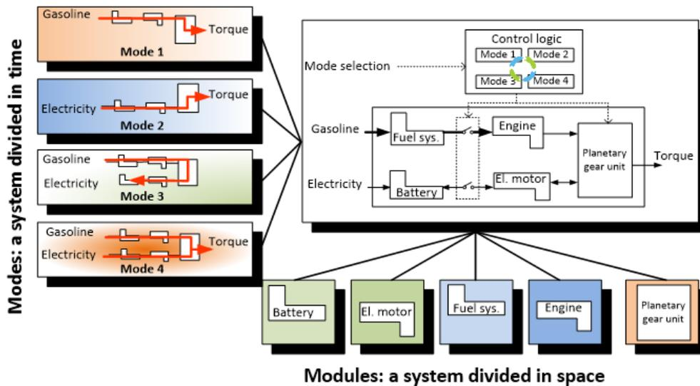
Figure 3. The physical configuration of a hybrid drive train divided in time and space
