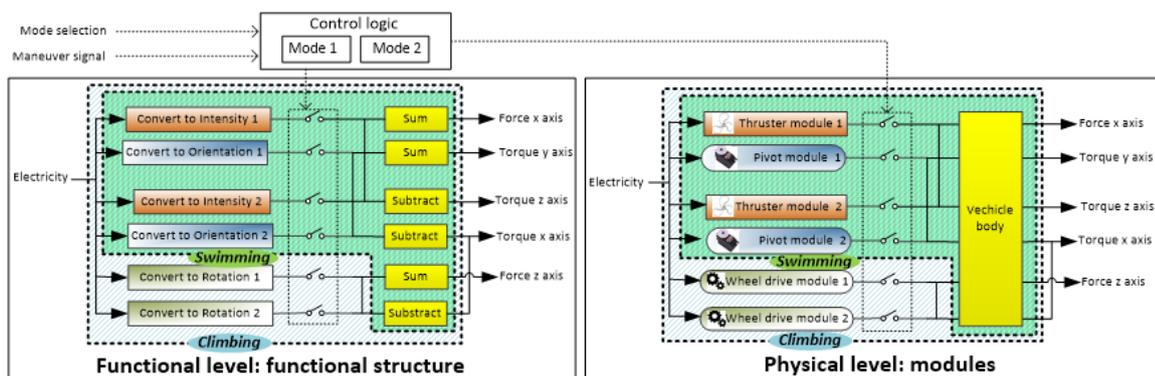
Figure 7. The modular architecture of the Searazor prototype
