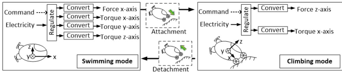
Figure 4. The major functions of the two-mode underwater vehicle
