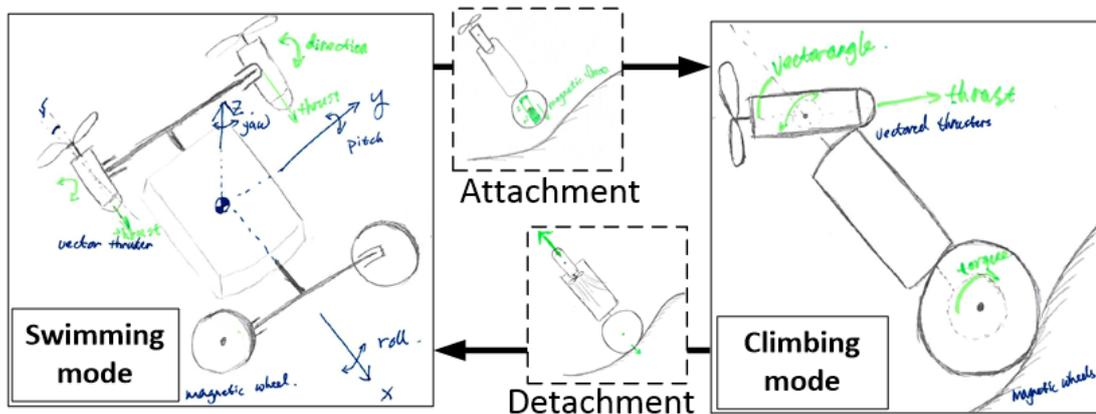
Figure 5. The concept of the Searazor swimming-climbing underwater vehicle
