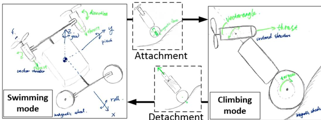
Figure 5. The concept of the Searazor swimming-climbing underwater vehicle
