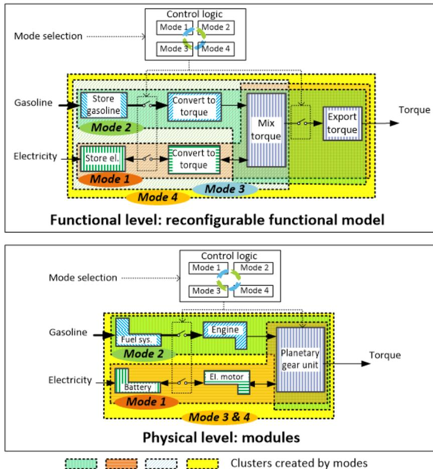
Figure 2. Product architecture of a hybrid drive train
