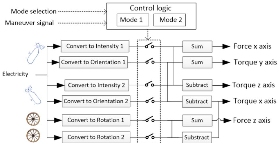
Figure 6. The reconfigurable functional model of the Searazor prototype
