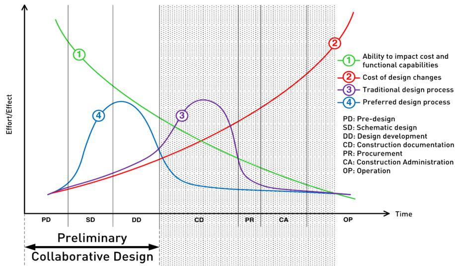
Figure 1. MacLeamy curve. A project that places significant efforts in preliminary design improve its cost-efficiency ratio.
