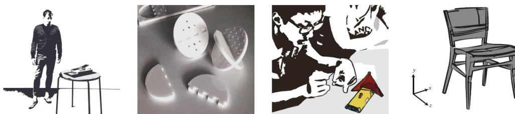
Figure 3. (left to right) scaled prototype (architectural), isolated subsystem (simple joints), relaxed requirement (paper mockup), virtual prototype (chair aesthetic design)
