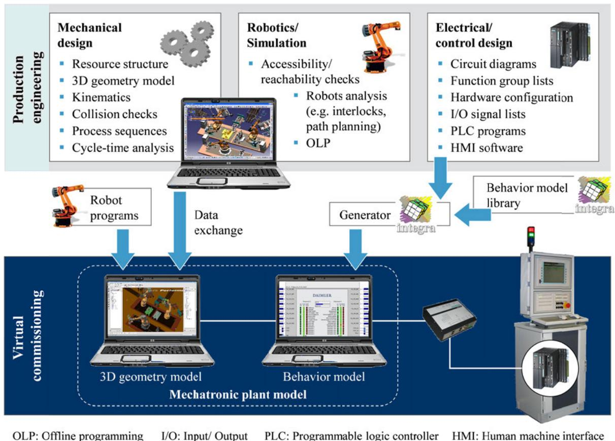
**Figure 3. Virtual commissioning – Data supply and workflow**
