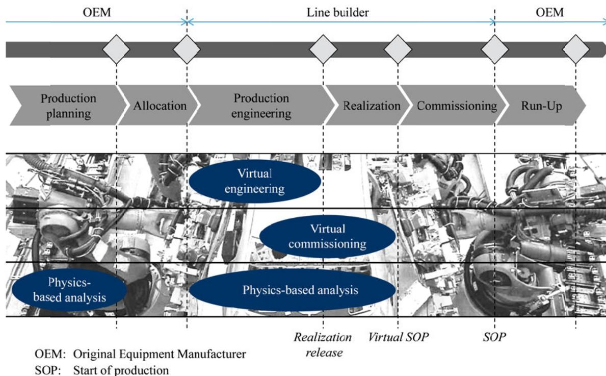
**Figure 1. Lean digital validation methods within the production creation process**
