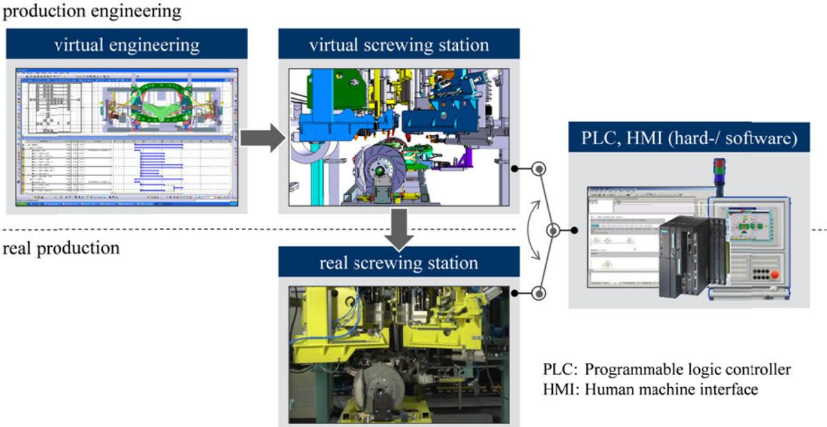
Figure 5. Operational application of virtual engineering and virtual commissioning
