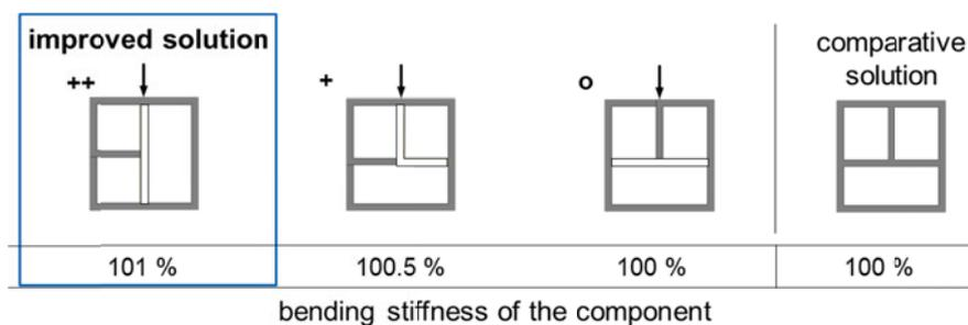
**Figure 11. Using returned cognition in designing the cross section of a bending beam**
