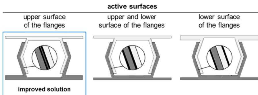
**Figure 12. Using returned cognition in designing a snap connection**
