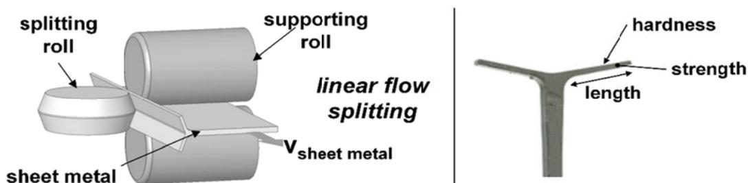
Figure 1. Linear flow splitting - process and product
