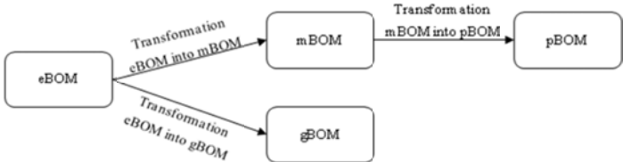
Figure 3. Concept of BOM transformation in BOM-centric PDM
