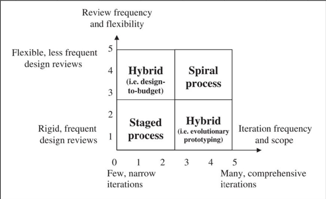
**Figure 1. PDP categories based on review and iteration characteristics [Unger and Eppinger 2011]**
