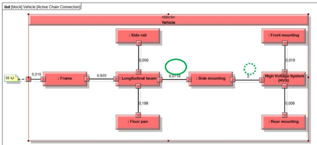
**Figure 7. Internal block diagram: New energy absorption ratios calculated for a new design concept (parametric solver) (values added to the figure for comprehension)**
