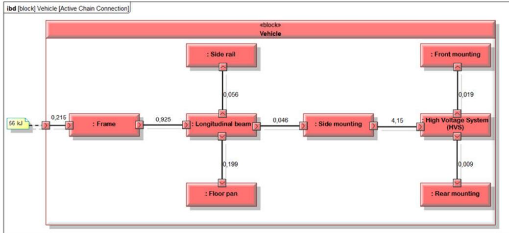
**Figure 6. Internal block diagram: Energy transfer of the load path (pole side impact) in a block definition diagram (proportional values added for comprehension) based on a vehicle crash simulation**
