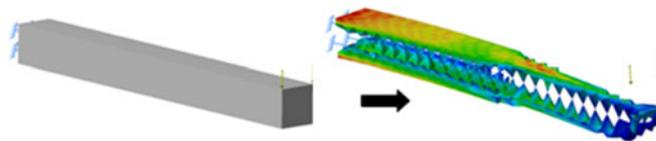
**Figure 3. Topology optimization using the example of a simple beam**
