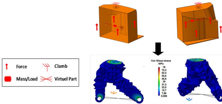
**Figure 8. Result in post-processing of the topology optimization mounting design space with a load in x-, y -and z- direction**
