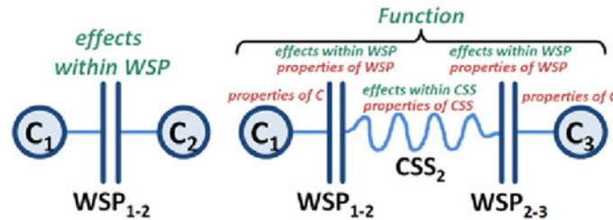
**Figure 1. "Effect" and "Function" in the C&C<sup>2</sup>-Model based on the C&C<sup>2</sup>-A [Zingel et al. 2012]**
