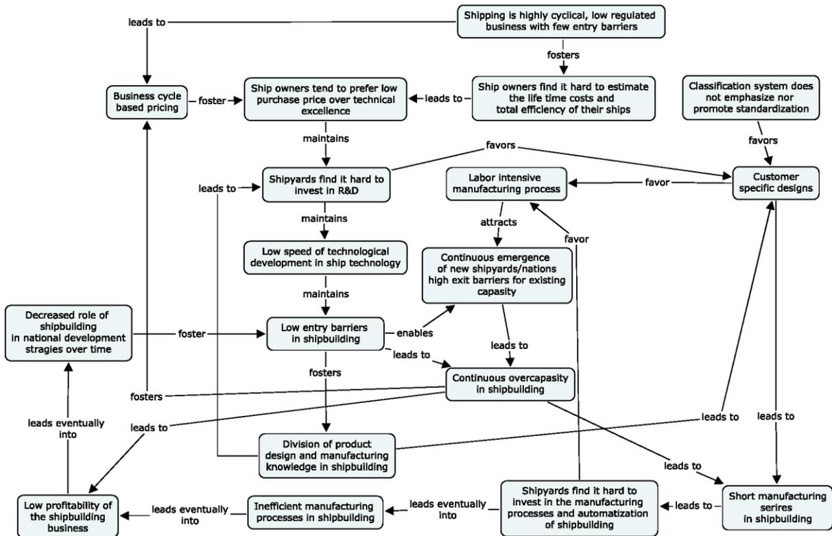
Figure 1. Concept map representing the factors with effect of engineered-to-order (ETO) industrial paradigm in shipbuilding industry.
