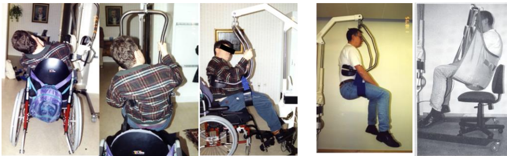
Figure 6. Universal person lifting aid to be used instead of slings (the far right picture). To the left is shown the lifting of a disabled person from a wheel chair. The fourth picture shows a person being transported with a mobile lift from one place to another.
