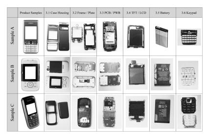
Figure 3. Product Sample Study of a mobile phone (Major modules of sample A, B and C)
