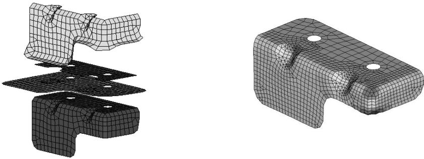
**Figure 1.** Thinning contour plot from LS-DYNA showing 19.5% thinning at the corner of the formed part (blank) [25].
