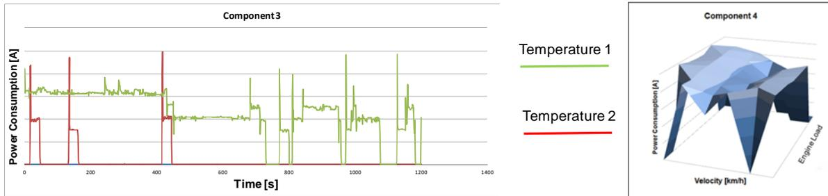
**Figure 9. Dependencies between component 3 and temperature (left), dependencies between component, velocity and engine load (right)**
