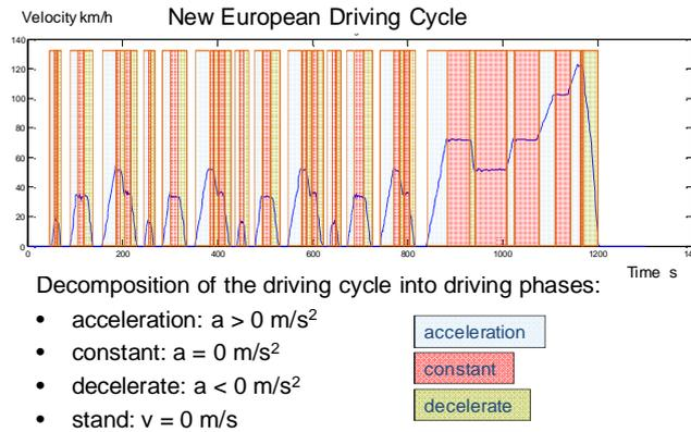
**Figure 6. Decomposition of a driving cycle**
