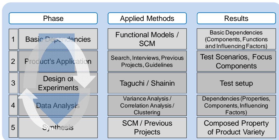
Figure 3. Procedure model supporting validation for complex products
