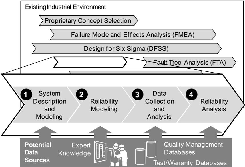
Figure 2: Early reliability prediction method embedded into the industrial environment
