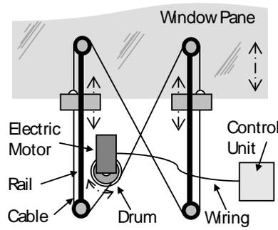
Figure 8: Sketch of a double-rail drum and cable window regulator
