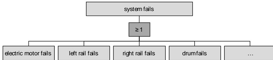
Figure 9: Fault tree combining component failures to system failure
