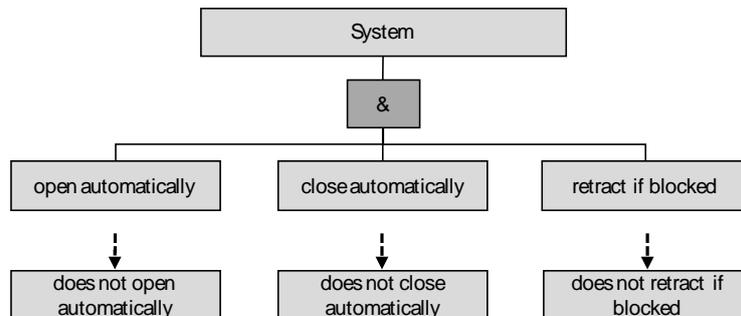
Figure 7: From the function tree of a Car Power Window Regulator, malfunctions can be deduced
