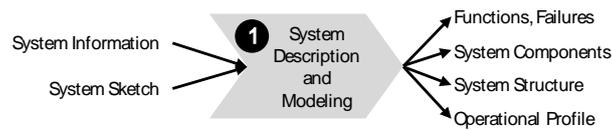
Figure 3: Phase 1 - System Description and Modeling
