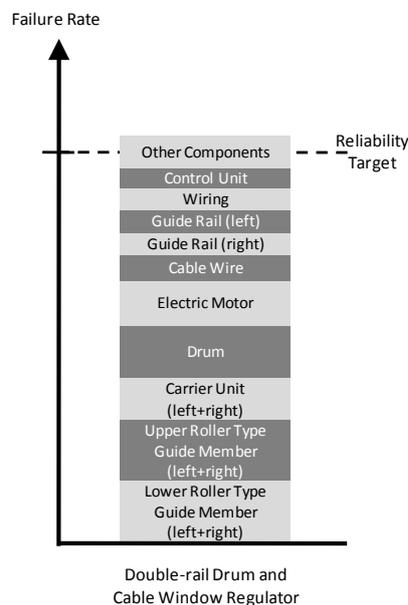
Figure 10: Failure rates summed up and compared to the reliability target
