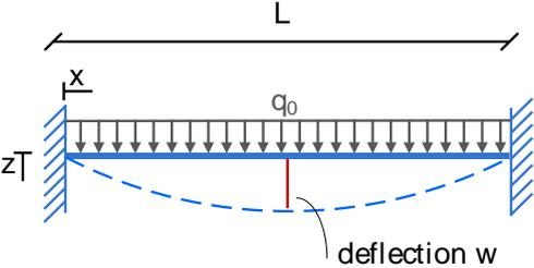
Figure 7: Abstraction of the chamber wall to apply beam theory
