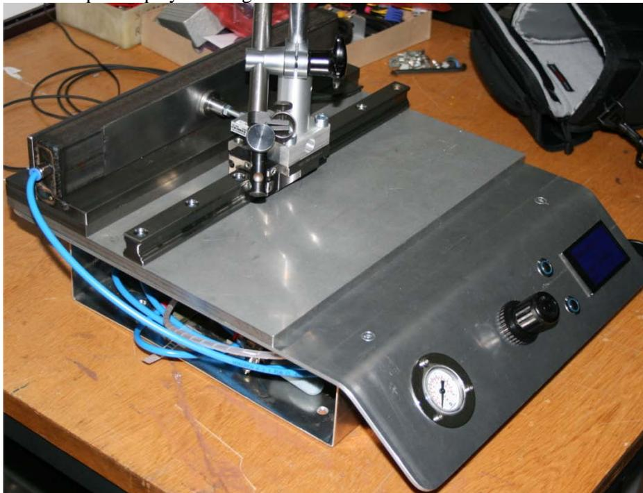
Figure 9: Test setup to measure force and deflection during inflation
