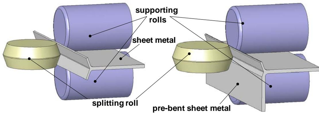
Figure 1: Schematic of the linear flow-split and linear bend-split processes
