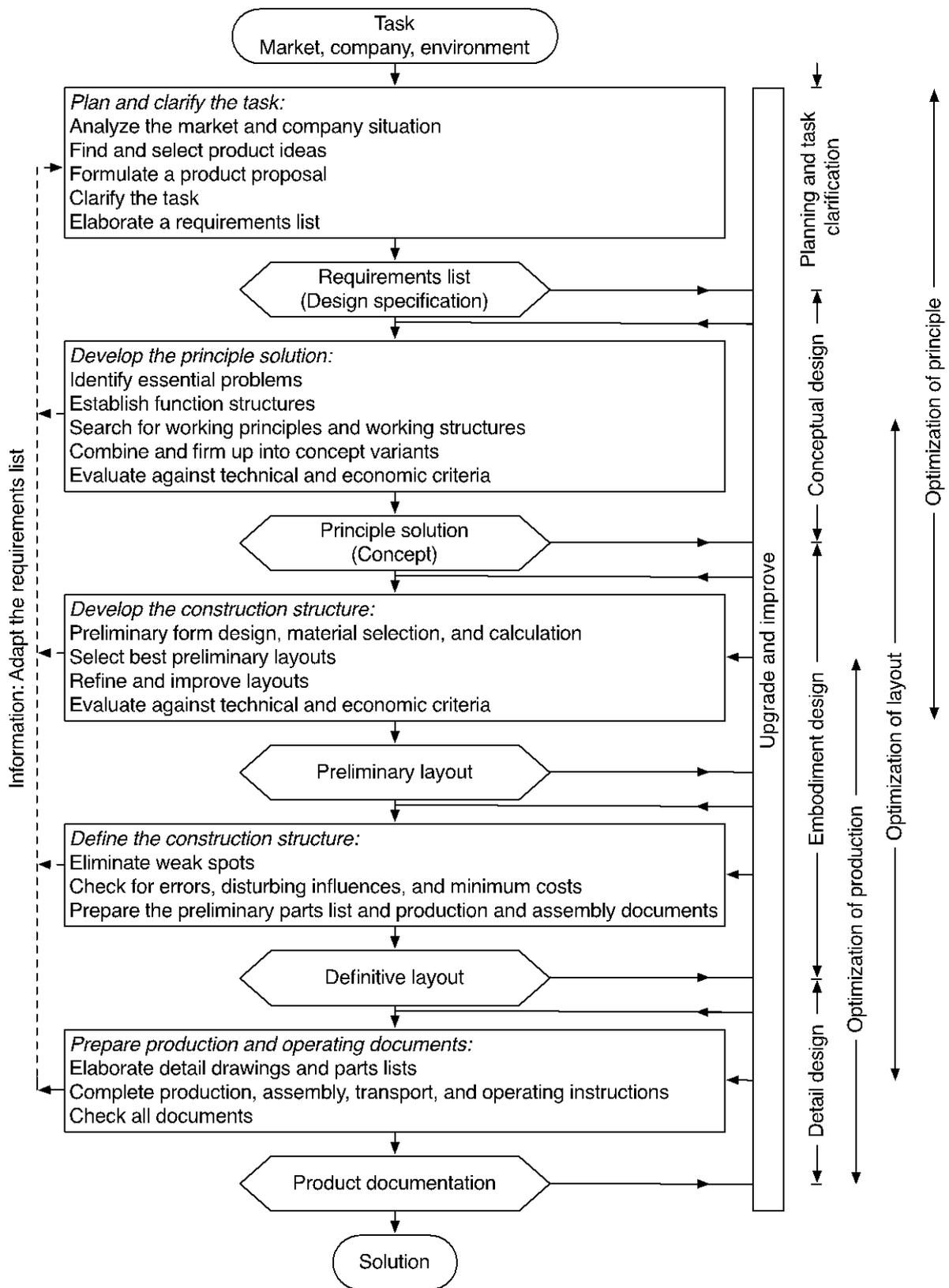
Figure 4 – Steps of the planning and design process (SPDP) [13]
