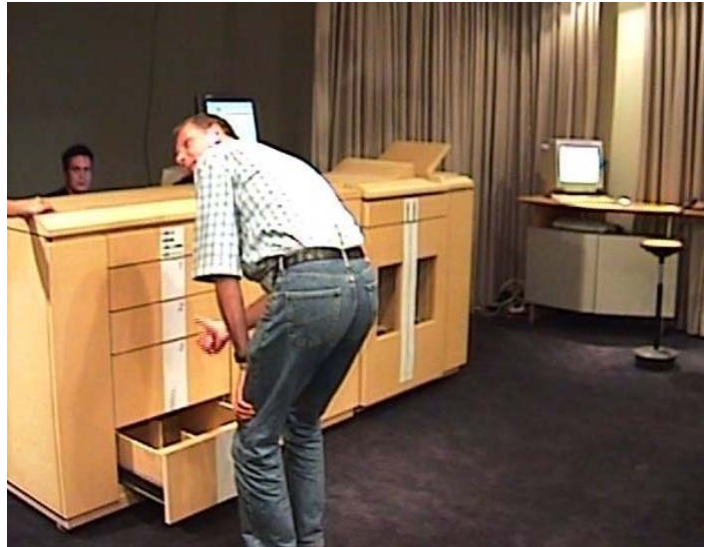
Figure 3: A usability test in the early phase of a project. The intended product is mimicked, including sound, and behavior of the product. A test person pressed a 'button' to open a paper drawer which was opened manually by a team member in the back.
