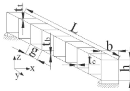
Figure 1b. Sandwich panel modeled as a beam
