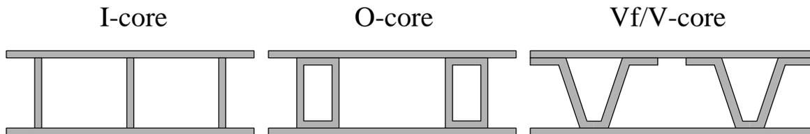
Figure 2. Typical steel sandwich panel cross sections
