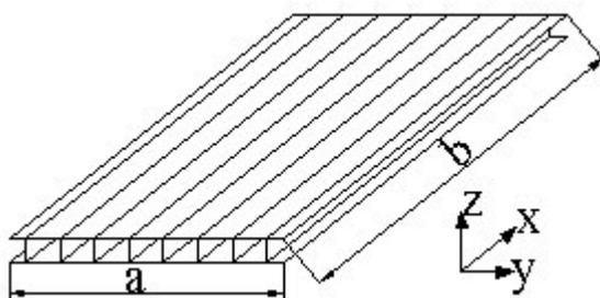
Figure 1a. I core all steel sandwich panel
