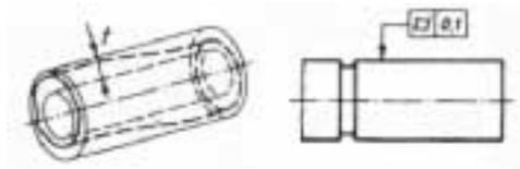
**Figure 9. Cylindricity tolerance**
