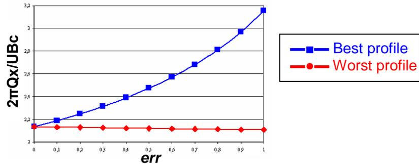
**Figure 14. Tolerance Abacus: circumferential flow as function of  $err$  for a fixed Sommerfeld number  $1/\Delta = 0.2$**
