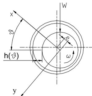
**Figure 2. Reynolds equation parameters in the journal – bearing kinematic joint**
