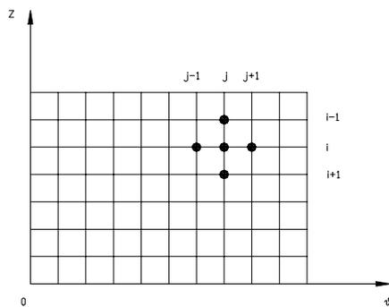
Figure 3. Finite difference mesh
