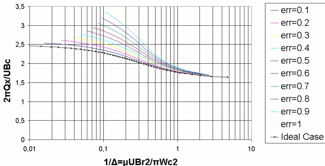
**Figure 13. Circumferential oil flow as function of the Sommerfeld number for several tolerance values**
