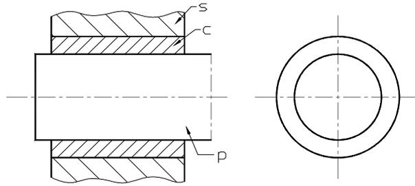
**Figure 1. Journal – Bearing kinematic joint**
