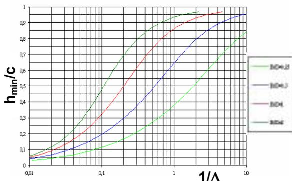
**Figure 7. Minimum thickness of the film**
