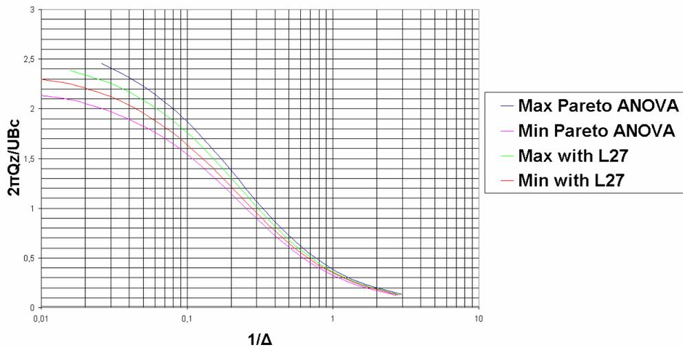
**Figure 12. Additive model validation: Axial oil flow as function of the Sommerfeld number**
