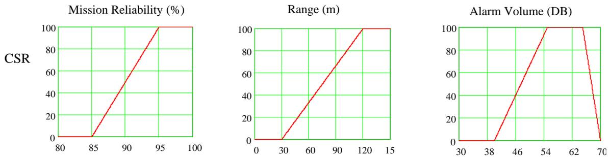
**Figure 3. Sample of system CSR functions: Mission Reliability, Range, Alarm Volume**
