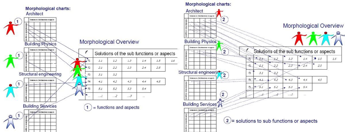
**Figure 3. Building the morphological overview; Step 1; The Morphological overviews show the agreed functions and aspects (1) of the different morphological charts. Step 2: The Morphological Overview with the agreed on sub solutions (2) from the separate morphological charts**
