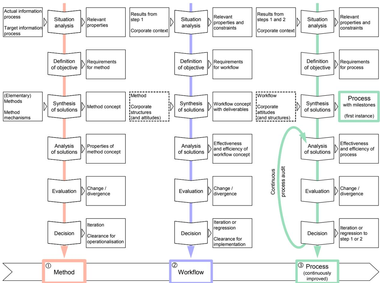
Figure 4. : Methodology of Systematic Process Engineering [WEI-04]
