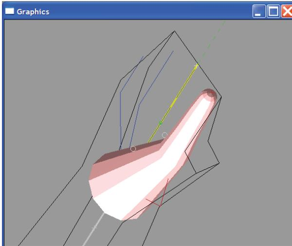
Figure 3 Surface descriptions of fingers using facetted spherical and conic models
