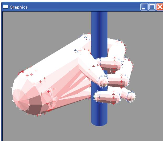
Figure 8 Multiple finger contacts around a smaller cylinder results in handrail type grip.
