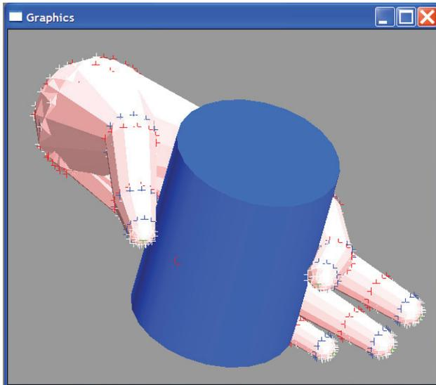
Figure7 Tip contacts around large cylinder generates cup-like grip.
