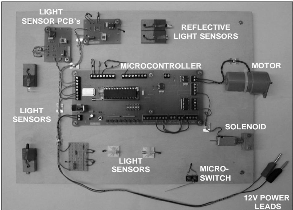
Figure 2. A microcontroller connected to a selection of actuators and sensors
