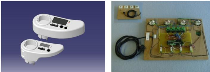
**Figure 3. Form prototype of integrated cognitive sockets (left) and functional prototype of cognitive power strip (right)**
