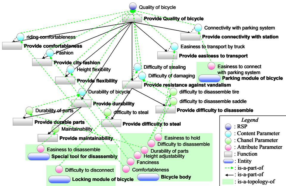
Figure 6. Service Engineering's view model of functions, channels, content and receiver state parameters (RSP) in the case of a bicycle rental service [Sakao 2006]
