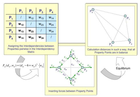
Figure 1. Approach by the forces model [Bauer, Meerkamm 2007]
