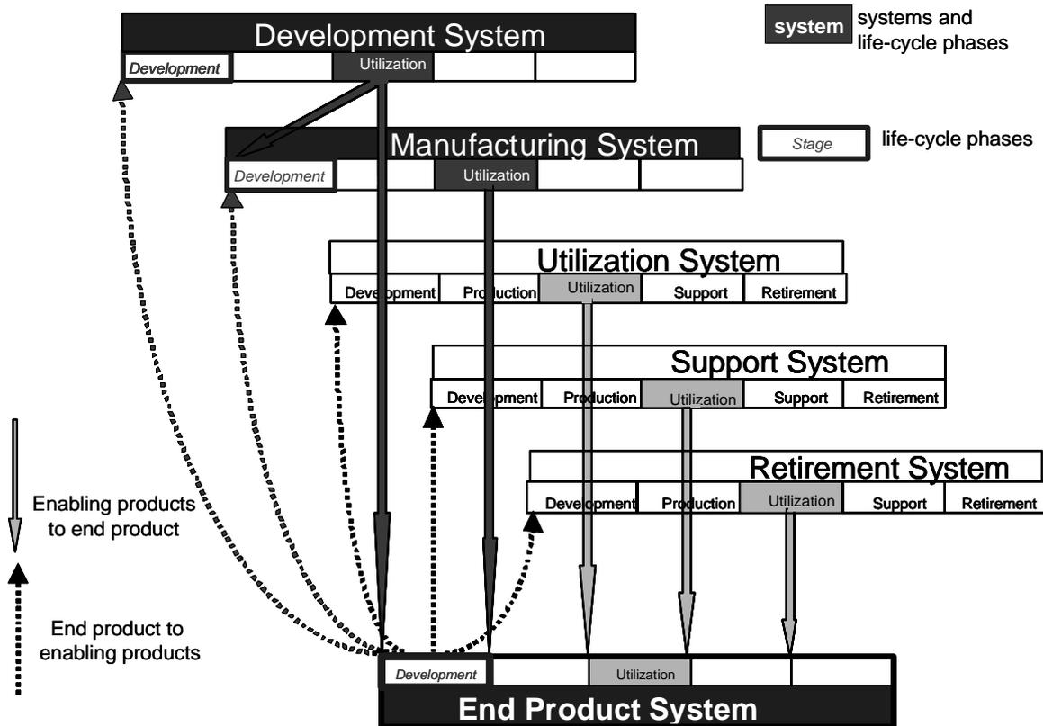
Figure 4. Links between the design system and the end product system adapted from [9]
