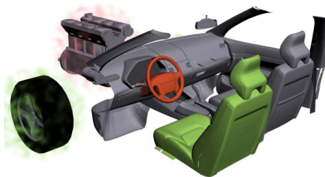
Figure 10. Illustration of main causes of vibrations
