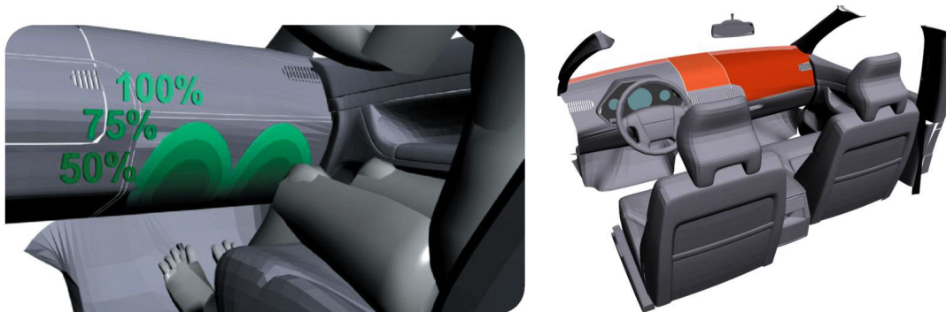
Figure 12. Likelihood of impact position for the knees. Color density as a result of potential weight reduction.
