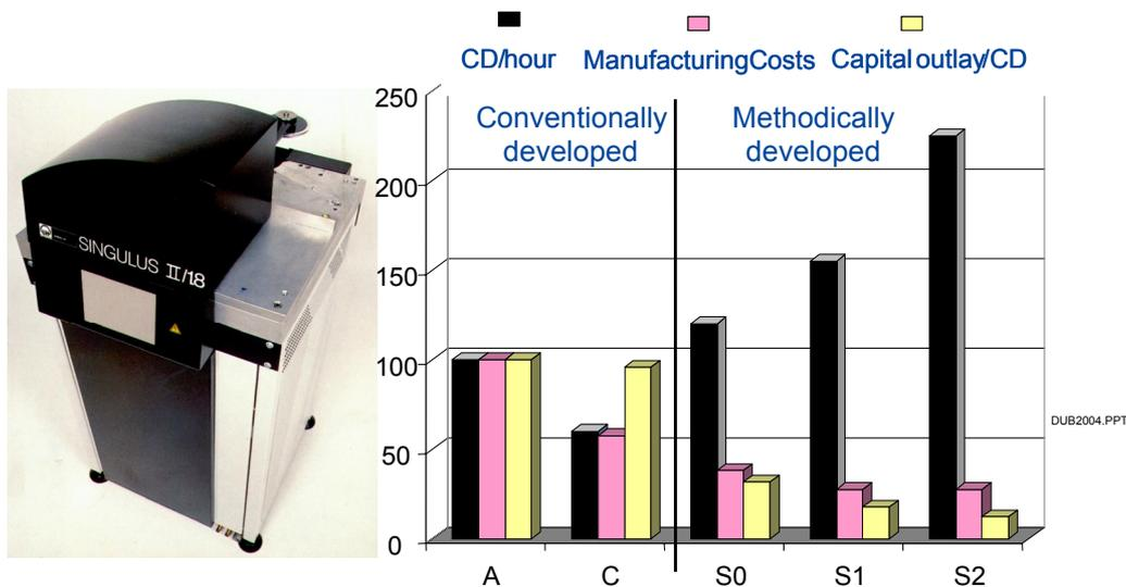
**Figure 5. The coating-CD machine and different steps of redesign**
