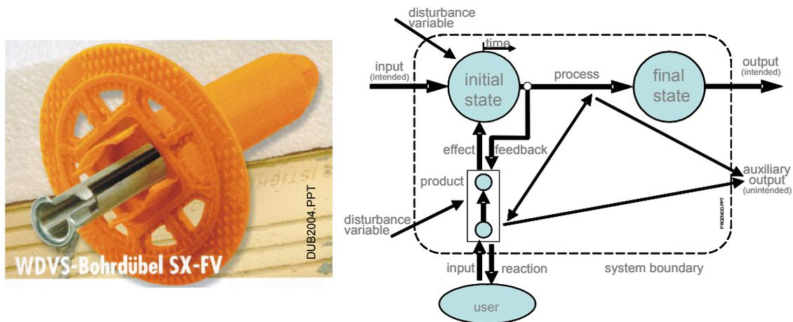
**Figure 2. The direct fastening dowel and the process model used for design**
