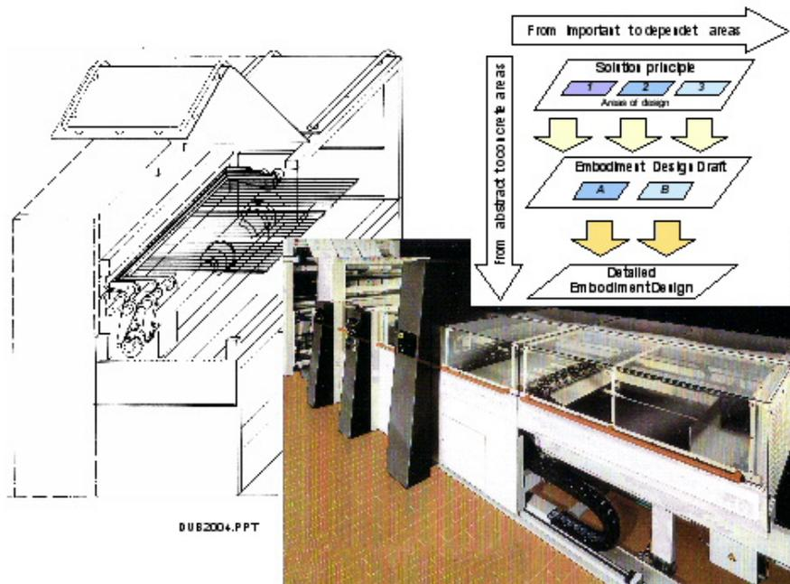
**Figure 4. The high-tech unit for stacking foil-bags – draft, embodiment design process, and unit, integrated in the final production equipment**
